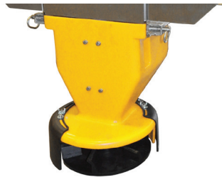
Spinner Chute – Forward handles and pins for easy on/off.
